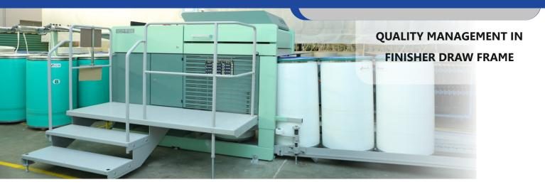
*LETER* D-50 Auto Leveller Draw Frame has a big influence on quality of the final yarn, because it is the last point in spinning to actually control and affect the quality.one of the main tasks of the draw frame is to improve the short-term and medium-term mass variation and linear density, with regard to evenness of slivers.
